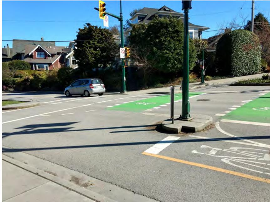
The intersection at Stephens Street and Point Grey Road has high visibility and clear direction of movement for all transportation modes, including a separate right and left turn lane for cyclists.
